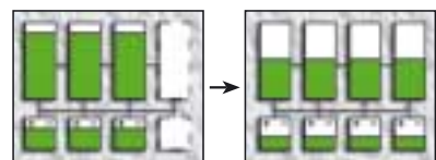
If three boards are not enough, fit an extra one. The load is automatically redistributed
