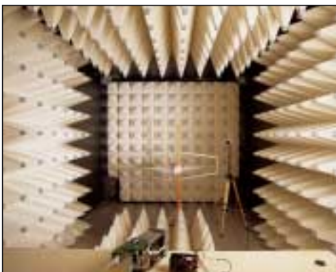
Anechoic room - R&D building
